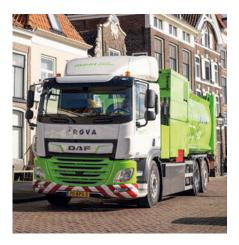
The City of London is by no means the only local authority to opt for electric RCVs. North London's Islington Council plans to deploy two later this year, while Sheffield City Council is already benefiting from a 2010-vintage Elite 26-tonner converted from diesel to battery power by Magtec; the first of two. Its useful life will be extended for several years; good news for the environment, and for the fleet's budget.
